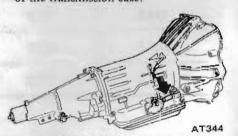
Fig. GI-9 Automatic Transmission Number Location
