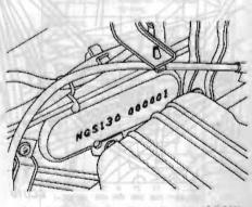
LC017 Fig. GI-2 Car Serial Number Location
