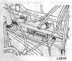
Fig. GI-4 Engine Serial Number Location
