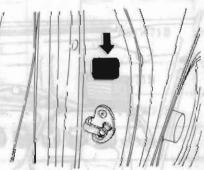
Fig. GI-6 F.M.V.S.S. Certification Label Location
