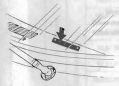
LC018 Fig. GI-3 Identification Number Plate Location
