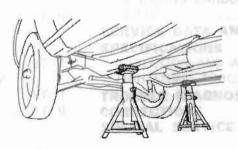
Fig. Gl-14 Front Supportable Points
