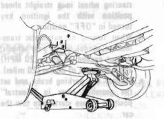
Fig. GI-13 Front Jack-Up Point
